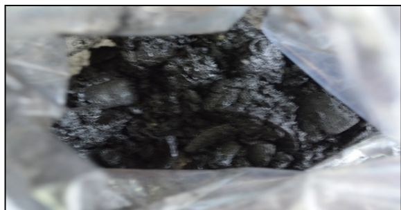
Fig-6: Debris collected after operations in well A
