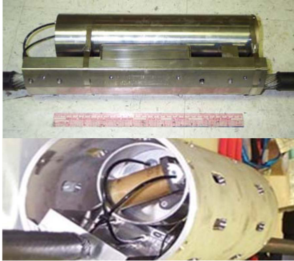
Figure 4. Sensor pad assembly showing a side view of geophone housing on sensor pad base (upper), and an end-on photo of the protective housing shows a hydrophone mounted in the pad (lower).
