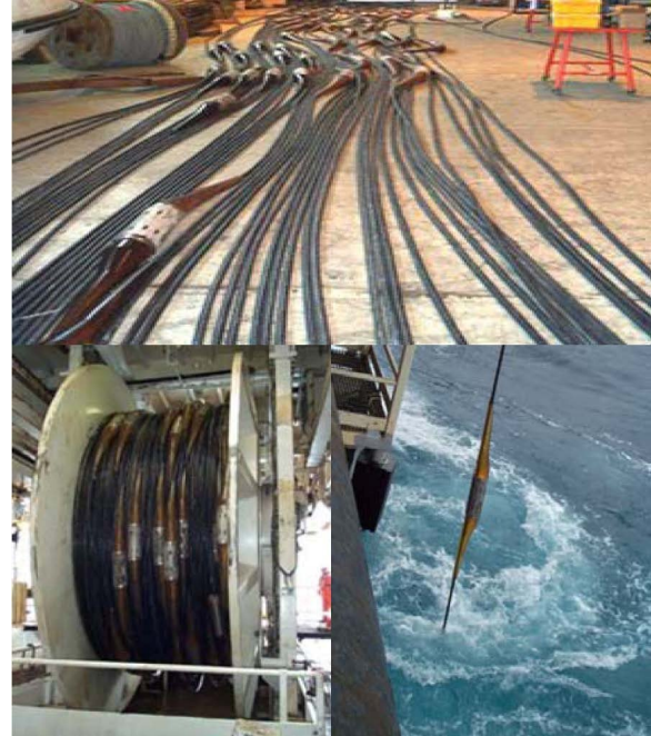
Figure 5. Optical seabed array being prepared in the warehouse (upper), on a deployment reel (lower left), and during deployed (lower right).
