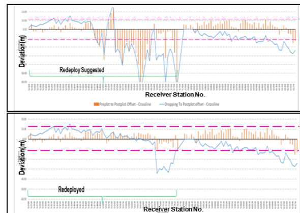
Figure 7: Crossline deviation (from preplot) histogram of a nodes line. Deviations before redeployment (Top) after redeployment (Bottom). The
