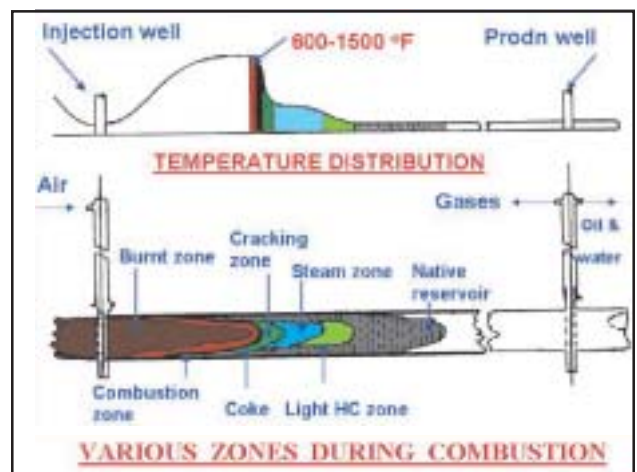
Fig.2: Schematic Diagram showing the principal of In-situ combustion.
