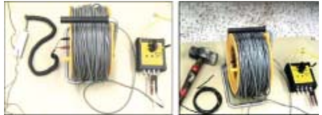
Fig. 2 : Interfacing for explosive & hammer
