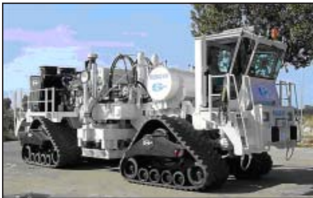
Fig. 3 : the Nomad 90T heavy vibrator (97,350 lbf) offers the highest mass-to-baseplate ratio (3.2 = 7.1 T / 2.2 T).
