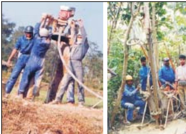
(a) (b) Fig 6: A & B type shot hole drilling rig.
