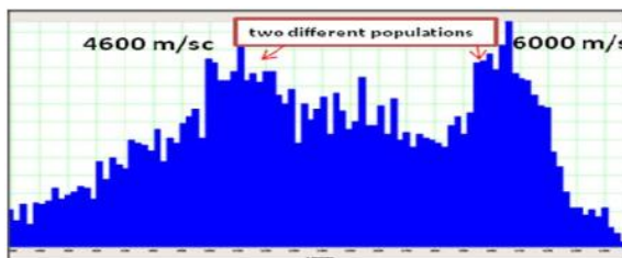
Figure 1(c): Histogram for P wave from the well showing two velocity populations at 4600 m/s and 6000 m/s.
