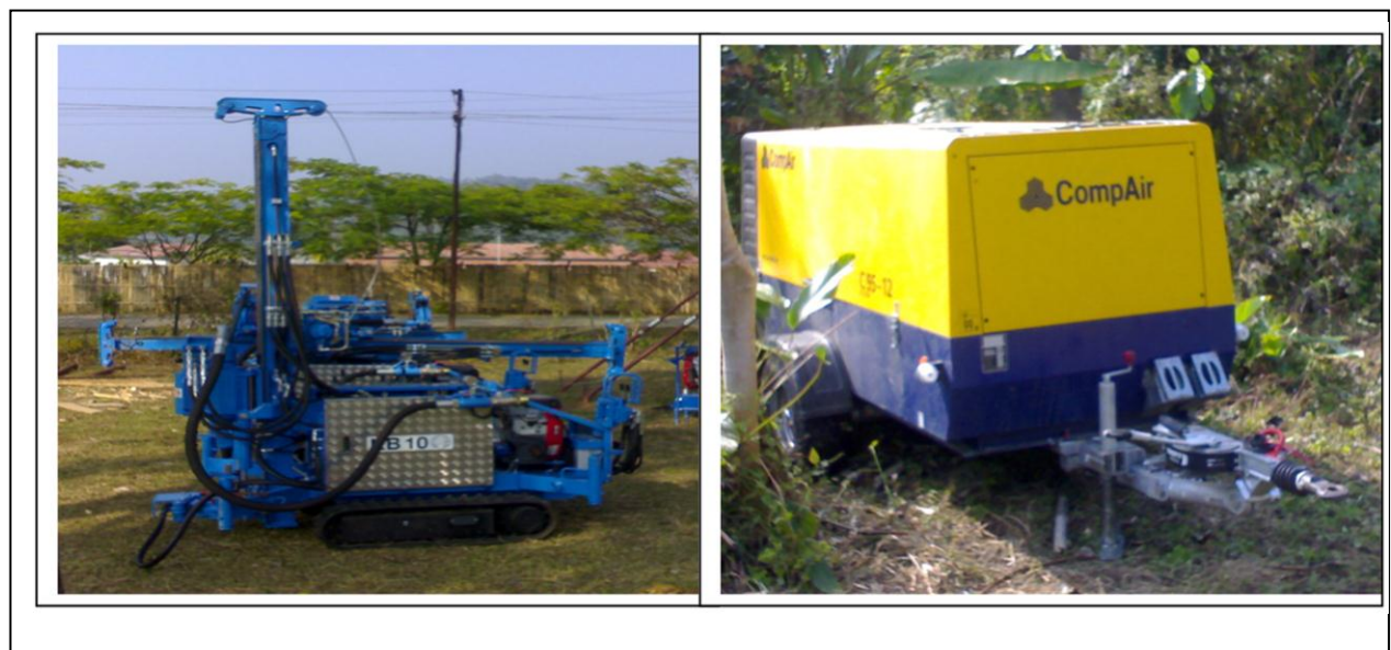
Figure 7 : KB-10 drilling rigs and the compressor (compare C-60)
